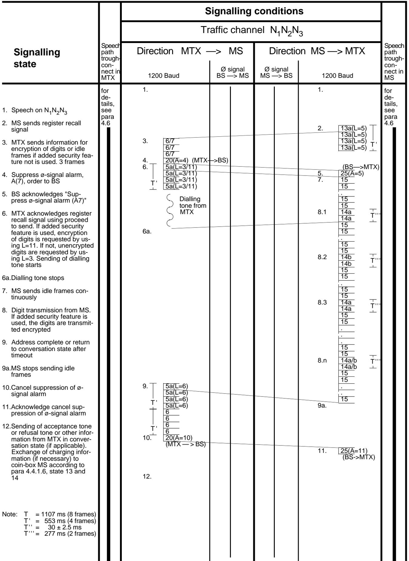
4.4.1.10.1b Optional use of register recall function, automatic transmission of digits
