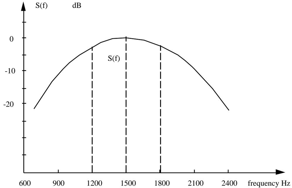
Fig. 4.6.4 Spectrum  $S(f)$  of the FFSK signal
