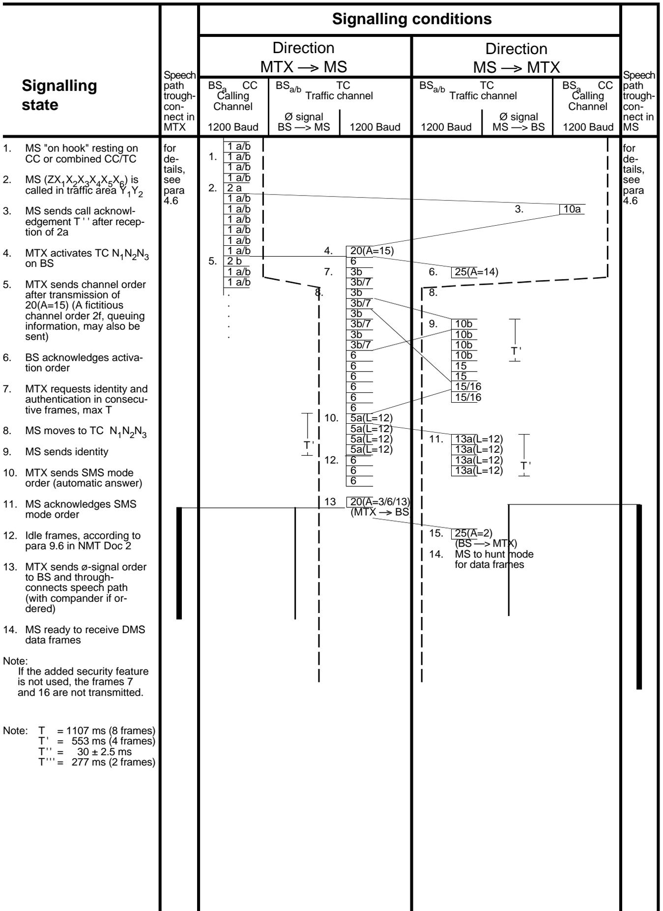
4.4.1.13 Call mobile telephone exchange to mobile station, with A-number and/or authentication **SCHEME B3** [optional]
