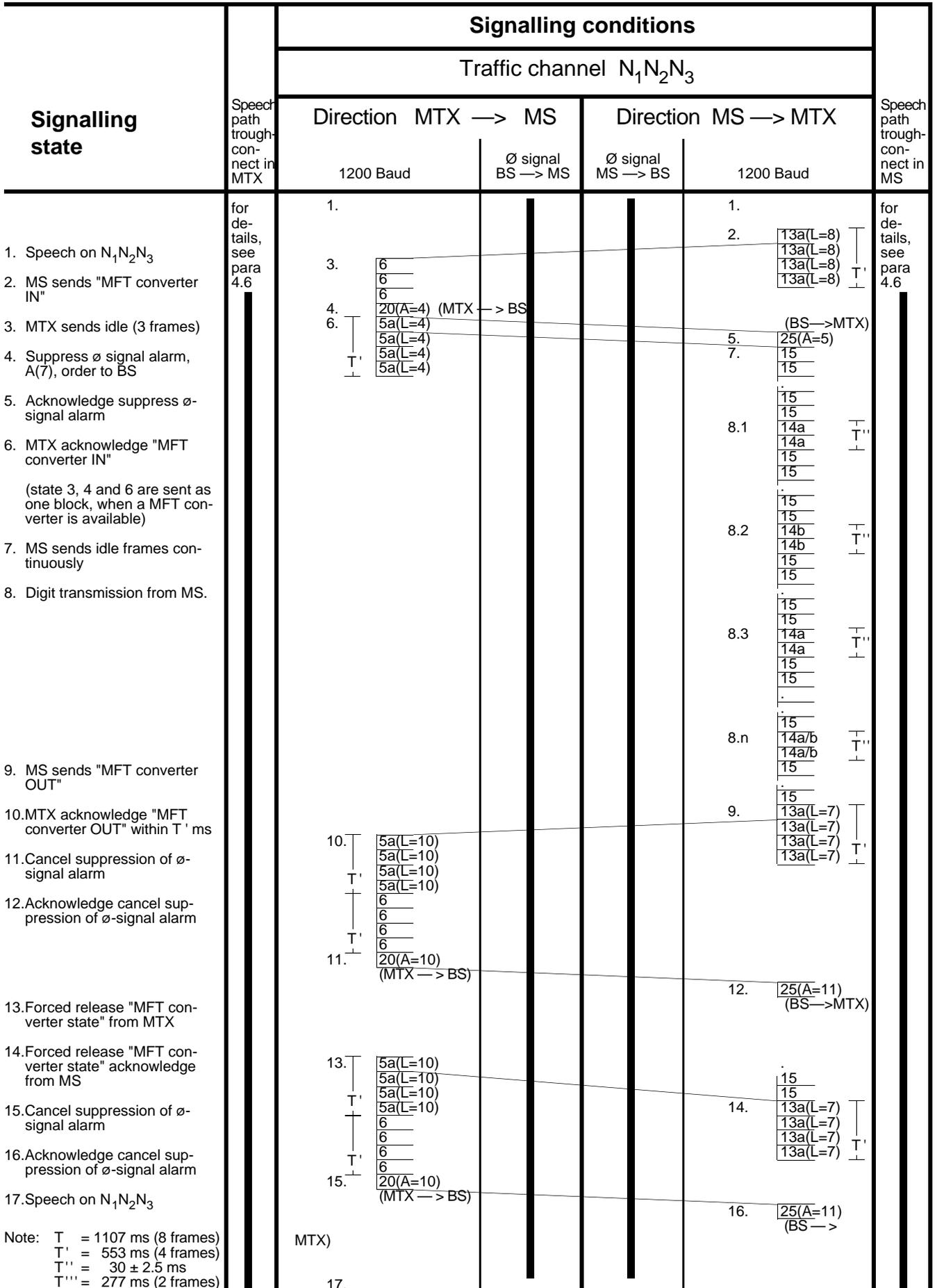
4.4.1.9b Optional use of MFT converter mode, automatic transmission of digits
