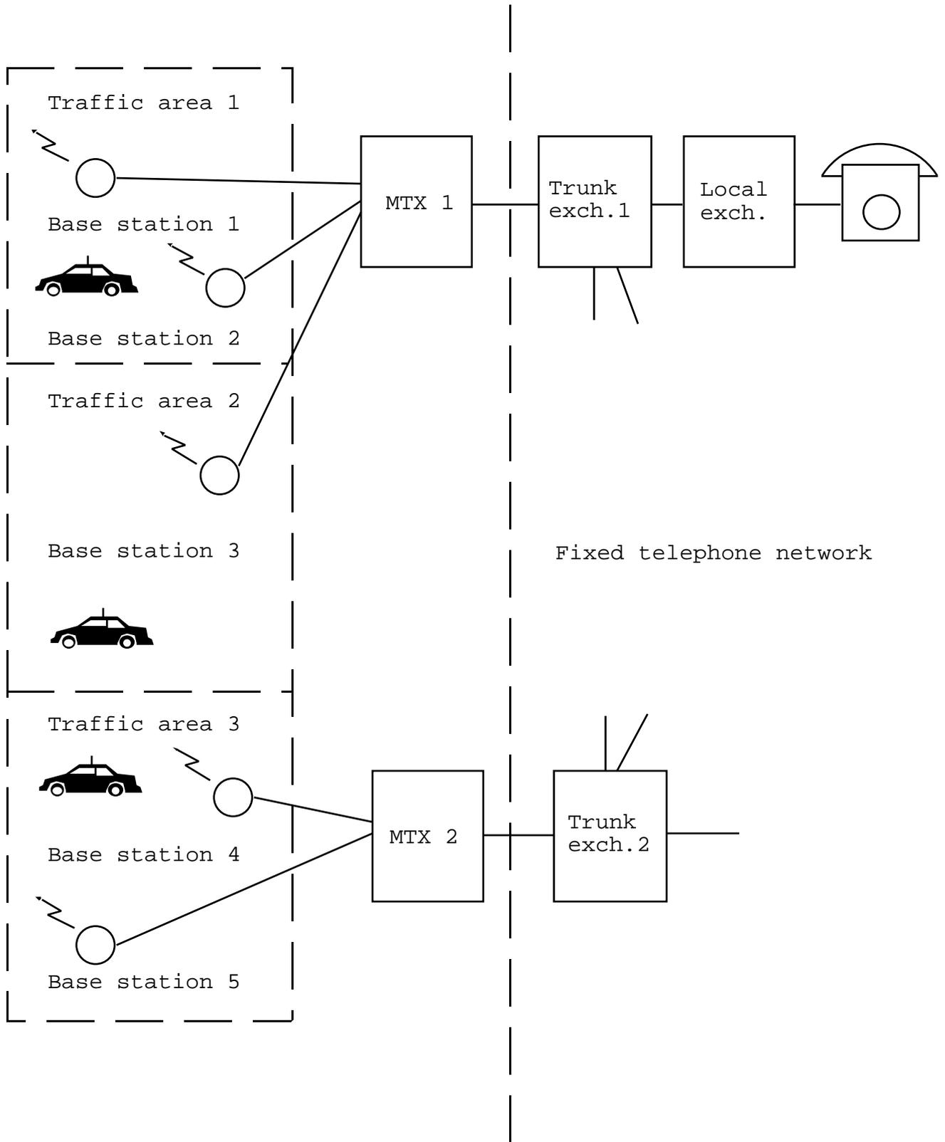
Fig. 2.1 SYSTEM STRUCTURE
