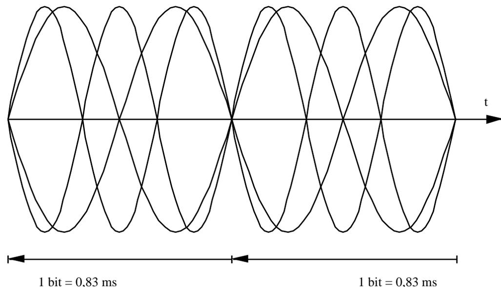
Fig. 4.6.3 Line diagram for the FFSK signal
