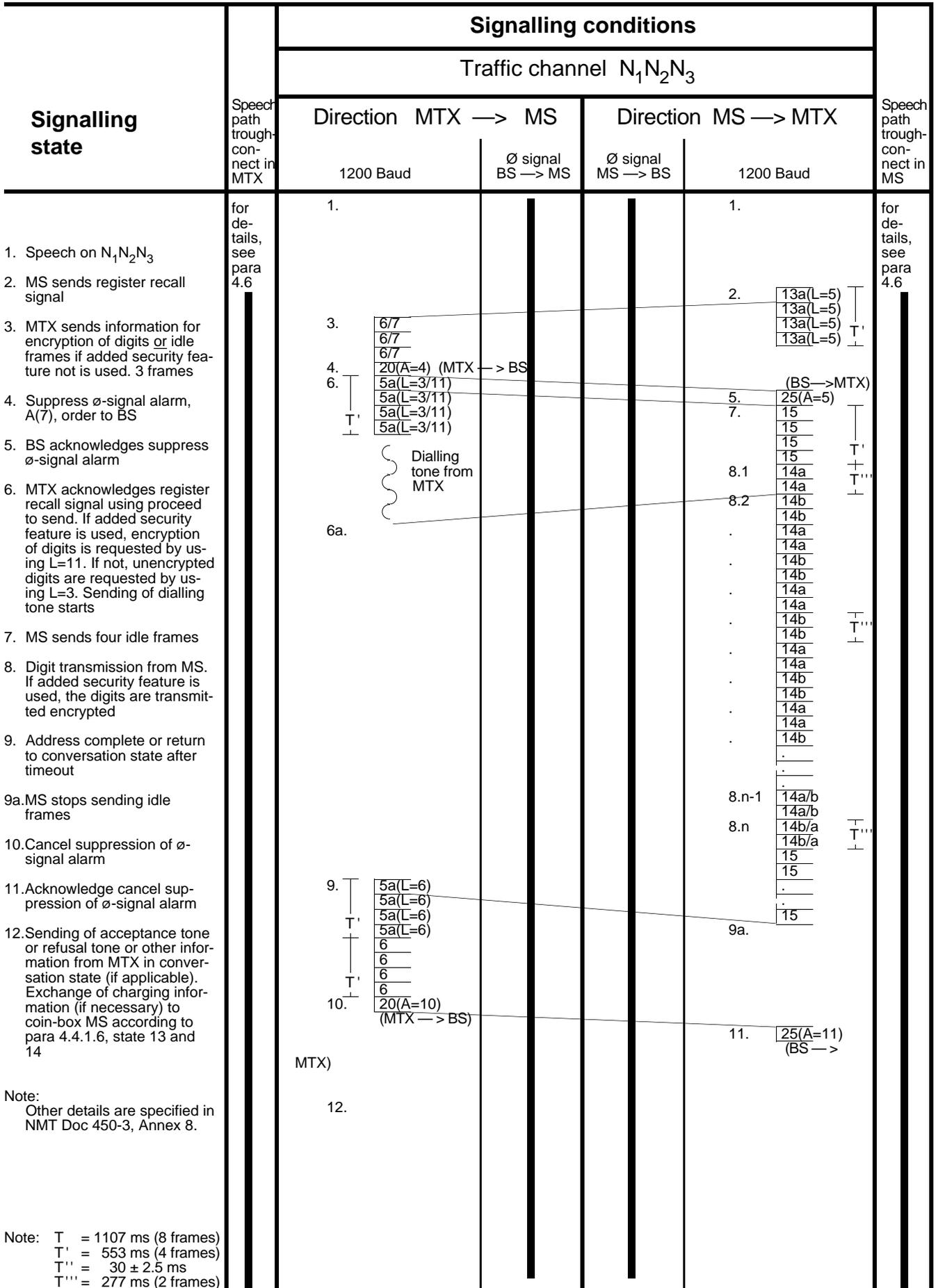
4.4.1.12 SMS call mobile telephone exchange to mobile station, normal case **SCHEME B2 [optional]**
